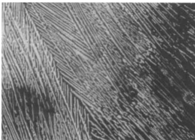
FIGURE 6 Dendritic finger like contours obtained for polyester PABO at 150°C on heating. (See Color Plate VI).
